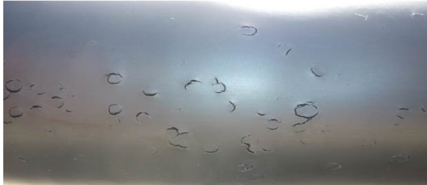
■ Figure 11. Cold Impact Damage Example
