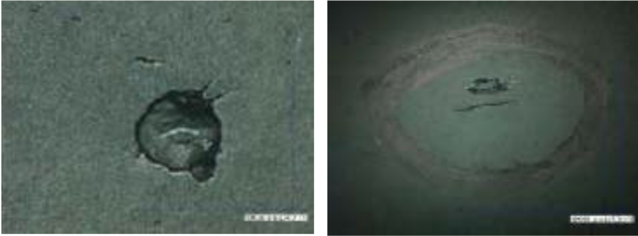
Figure 9. Pinhole caused by Static (left) or FOD (right)
