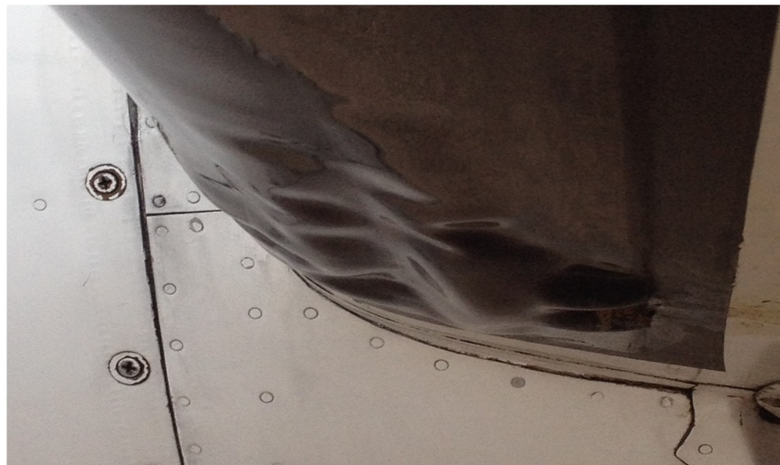
■ Figure 12. Fuel Contamination Example
