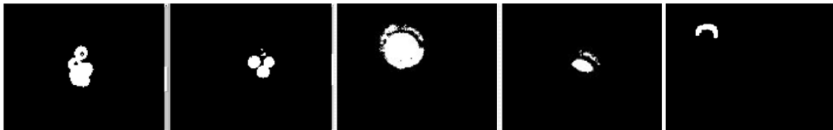
Figure 15. Pulse maps of various spot shapes used for spot-tracking firmware development.
