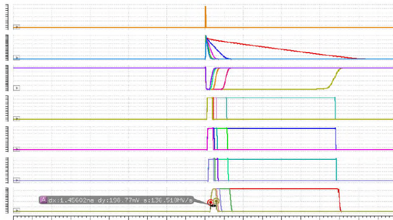
Figure 5: Simulated APD anode response Vs. quench voltage
