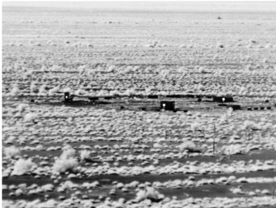
Figure 8: Low noise imaging (30fps) and the in-situ pulse detection of 3 separate laser sources using the same SUI MMT camera.
