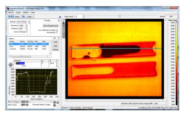
Line Profile: The ROI window graph on the lower left shows the pixel intensity profile along the horizontal green line on top of the image of the upper cuvette. This cuvette holds both water and used motor oil, while the lower one just has oil. SWIR imaging through a 1475 nm bandpass filter causes the water to appear black while the oil is red and airbubbles in yellow in this pseudocolorized image.
