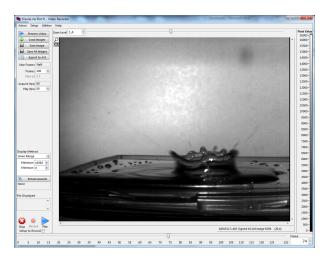
Video Recorder: The Video Recorder utility shows one frame of a video of water dropping onto a plate. The utility permits acquiring frames into computer RAM or to stream images onto media storage memory. Images can be recorded from the cameras at full speed and played back in slow motion, making use of all display and enhancement options. Frames can be stored individually or converted to a compressed AVI.
