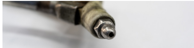
One 1/4-inch open nozzle used for employee cooling is roughly equivalent to 15 horsepower of compressed air.
