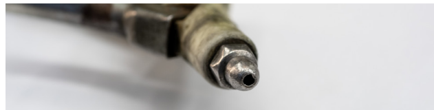
One 1/4-inch open nozzle used for employee cooling is roughly equivalent to 15 horsepower of compressed air.
