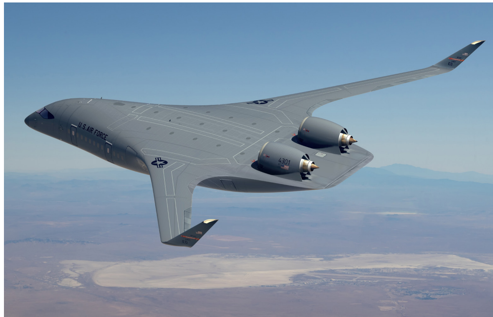
JetZero is developing its BWB concept for both military and commercial airline applications.
