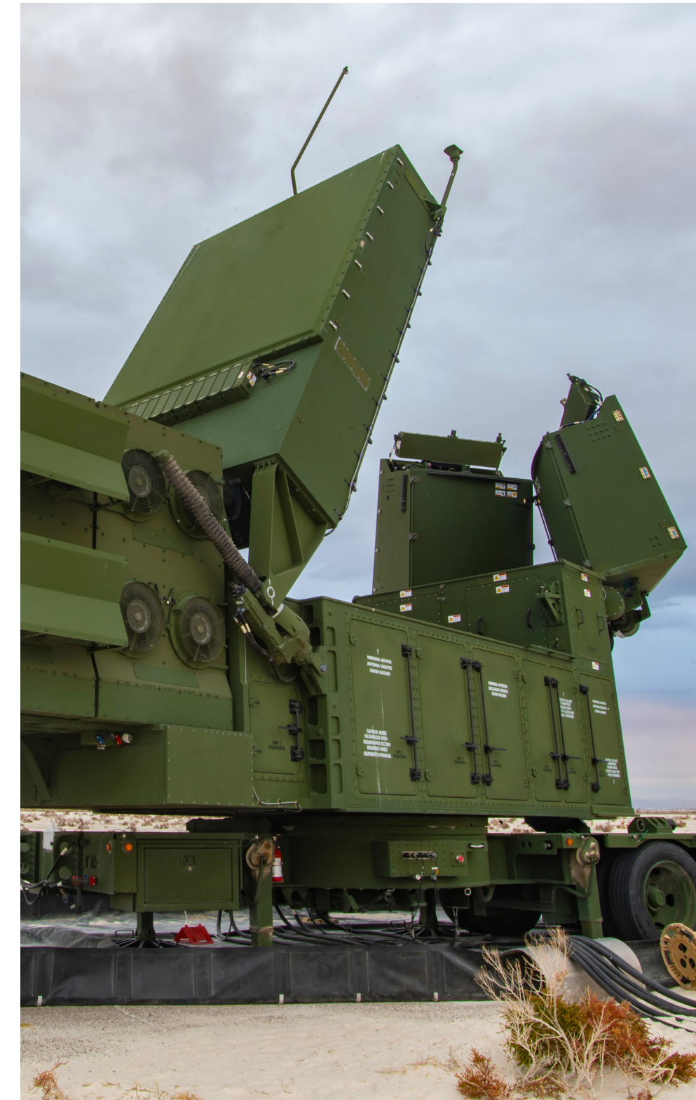
Raytheon designed its Lower-Tier Air and Missile Defense Sensors to be chromate free.
