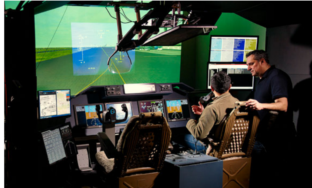
A Collins Aerospace reconfigurable flight deck display test platform, which enables tests to be conducted in an environment similar to that of actual flight before a system is delivered to the customer.
