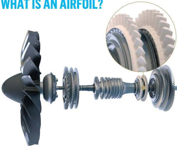
Turbine airfoils are an integral piece of the engine. Like a pinwheel, they spin the shaft that drives the fan and pushes the engine forward. They are small airplane wing shaped components that extract propulsive energy from the gas stream within the engine.
