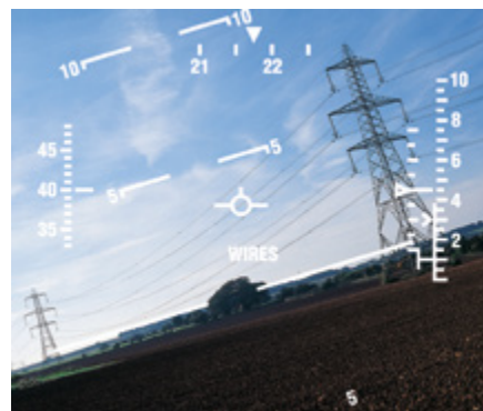
Wires warning and cueing
