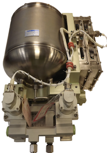
Pump and accumulator system for crewed capsule
