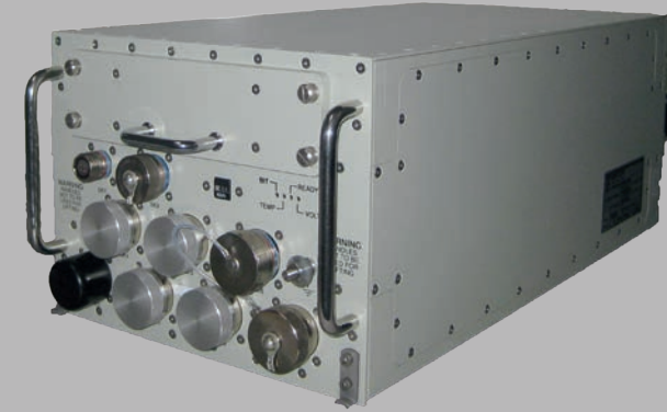
The DACAR Airborne Server incorporates the RABIT-N and SCi-Discover server technologies for in-flight data translation and data storage
