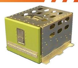
To remedy this situation, a filter is inserted into the recirculation duct, upstream of the recirculation blower fan. The filter is mounted inside an aluminum sheet metal box that is attached to the floor beneath the aft right hand seat. The filter element, which is designed to trap dust before it reaches the heat exchanger, can be removed periodically from the box for cleaning or replacement.
