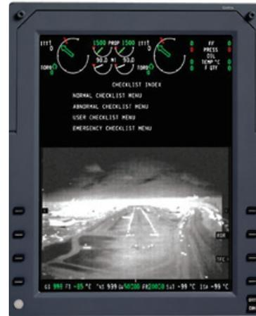
The display of video, in an NTSC format is presented on the lower half of the MFD. Video sources may be EVS, surveillance, or information cameras. Multiple video sources may be selected via an external switch.
