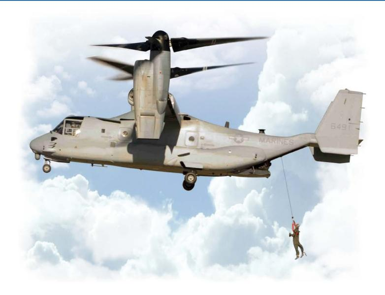
The 44312 Rescue Hoist is an internally mounted hoist and payout boom adapted from Goodrich 44311 series of external hoists. The rescue hoist is powered by the aircraft 115/200 VAC 3 phase 400 Hz power supply, and controlled with 28 VDC power.
