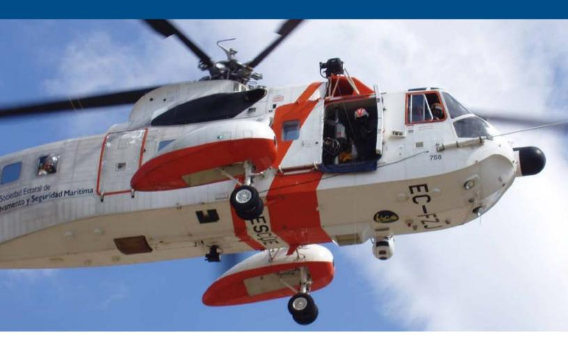
The externally-mounted hoist series 76378 are electrically powered and allow lowering and lifting operations under continuously variable speeds. By design, our hoists are simple in construction and incorporate a minimum number of piece parts, which makes them highly dependable, easy to maintain and reliable, with casing that provides a stiffness of the hoist.
