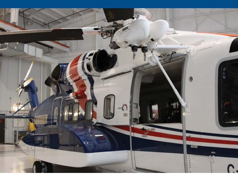
The 44311 series AC powered rescue hoist was specifically designed to meet the commercial performance specifications of the S-92, and has subsequently been adapted for installations on CH-47 and UH-60. The hoist design is also expected to satisfy the U.S. Army's strict electromagnetic impulse requirements defined in ADS-37. This commercial technology has been adapted for installation on the V-22.
