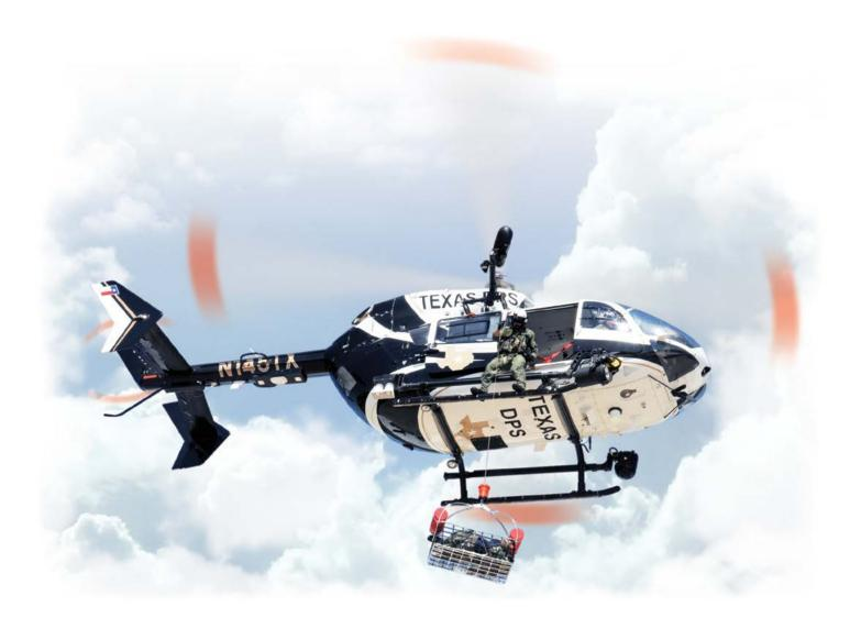
The 44301 series externally mounted 28 VDC electrically driven hoist incorporates all of the safety, self-sensing and redundancy features as well as the cable management system present in all other Goodrich category one hoist designs. These features enhance operational safety and unit reliability and extend the service life of the hoist assembly.
