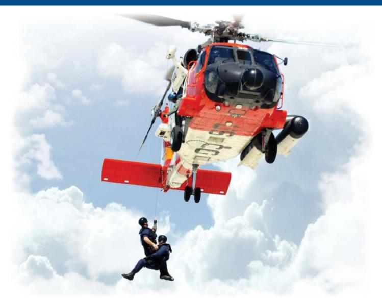
The 42315 series is a hydraulically driven, externally mounted hoist used for personnel rescue and other special operations. The 42315 series hoist has demonstrated high reliability, durability and reduced cost of maintenance through the years of operation with the United States Navy, United States Coast Guard, United States Air Force and international search and rescue operators.
