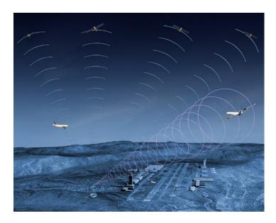
Multi-frequency/multi-constellation global navigation satellite system (MF/MC GNSS) capability is the future of global navigation. It provides SBAS-like precision and integrity anywhere in the world.
