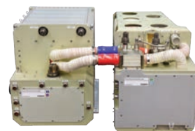
Thermal amine CO2 removal system
