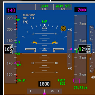
Current and next flap settings on airspeed tape with persistent "UP" indication
