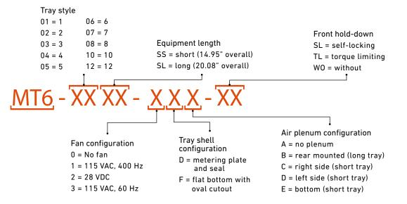
Contact us if fan or shock vibration isolators are required. We will generate a part number based on the configuration you select.
