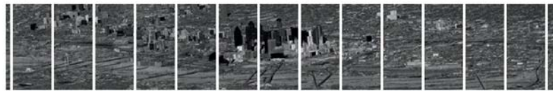
Section of 132 frames of dual band (EO/IR) mission task prior to panorama generation
