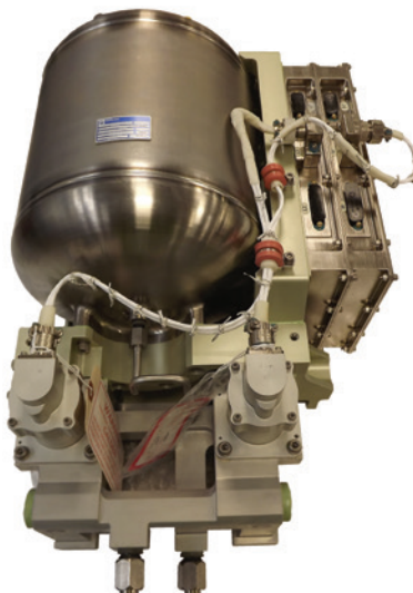
Pump and accumulator system for crewed capsule
