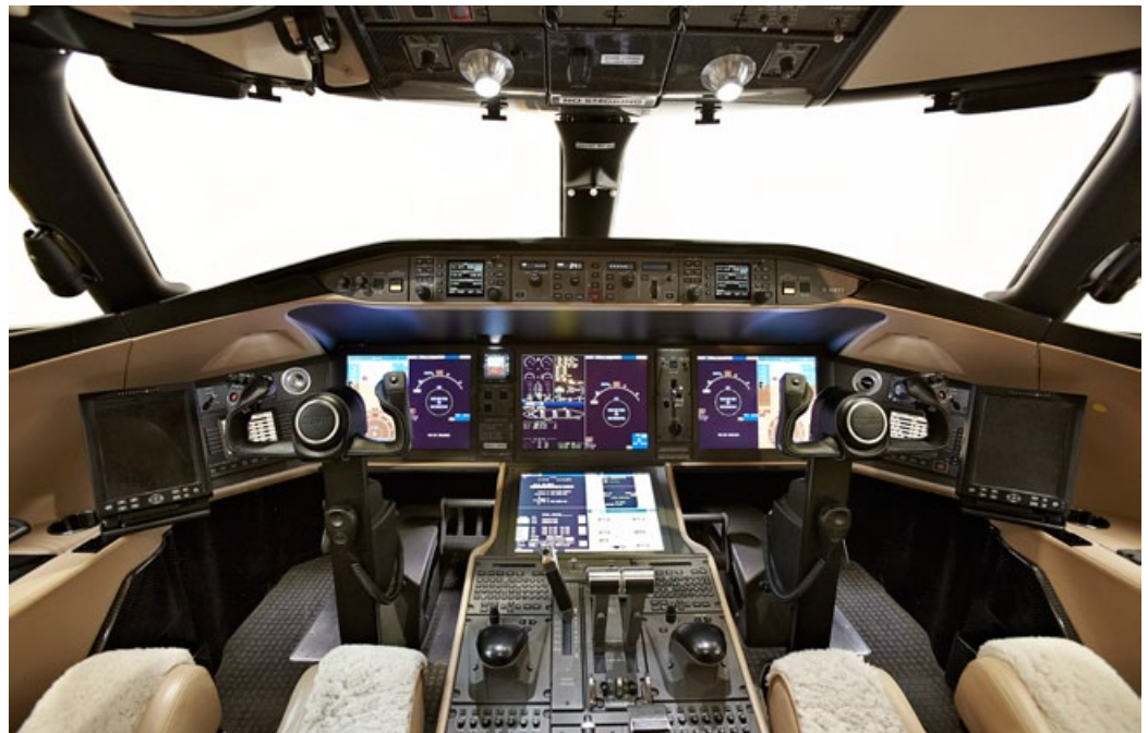
State-of-the-art LED technology on board the Bombardier Global 5000/6000: The Cockpit and Workstation Lights 2LA456026-00/-10 (see page 6) are mounted on the window frame to the left and right of the front pane.
