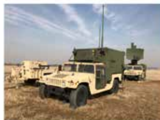
ATNAVICs operations shelter
