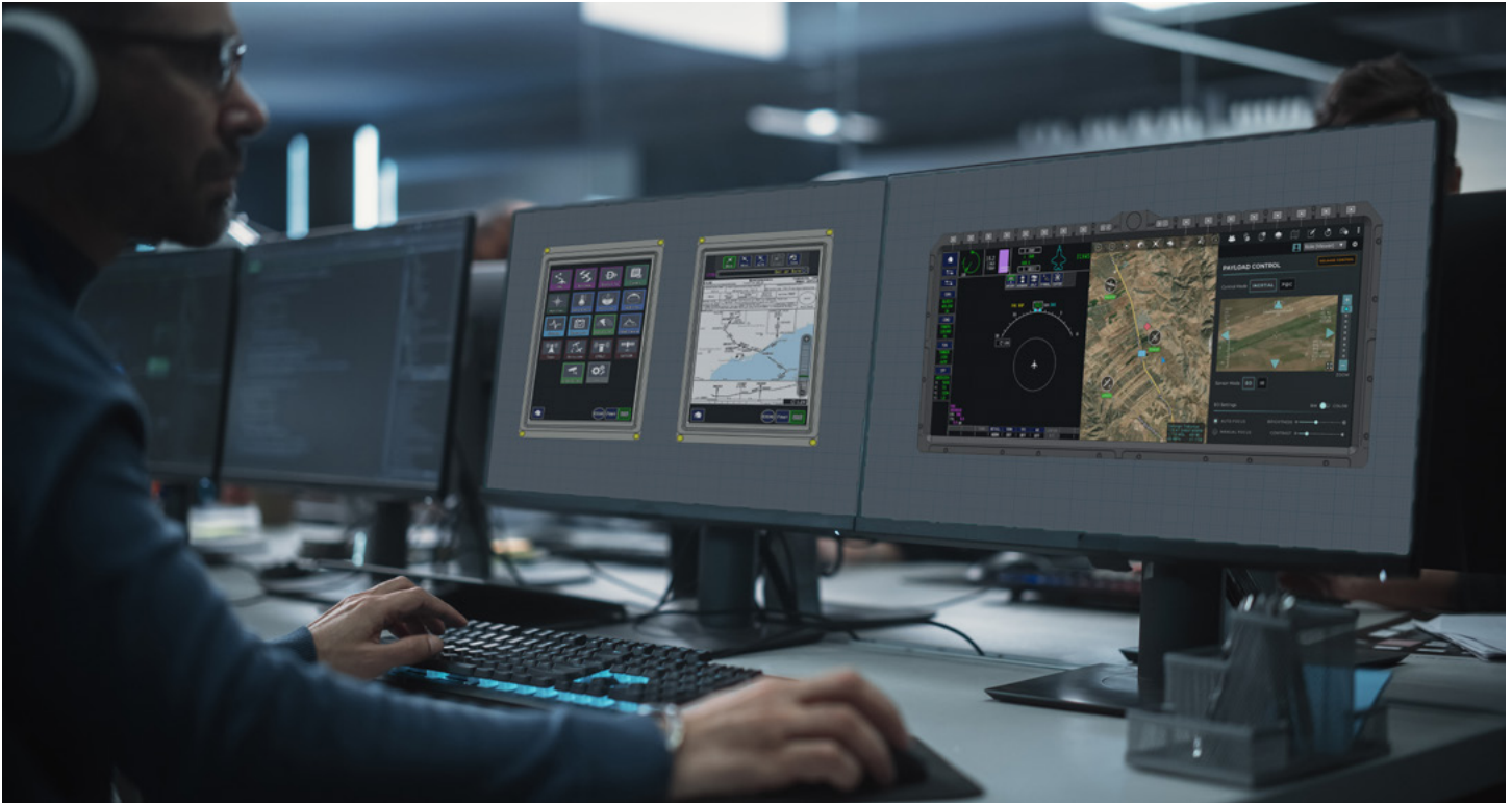
Figure 5 – Flight deck integrators are provided a combination of open APIs and plain-text configuration files to quickly incorporate new applications using their own development teams and tools.
