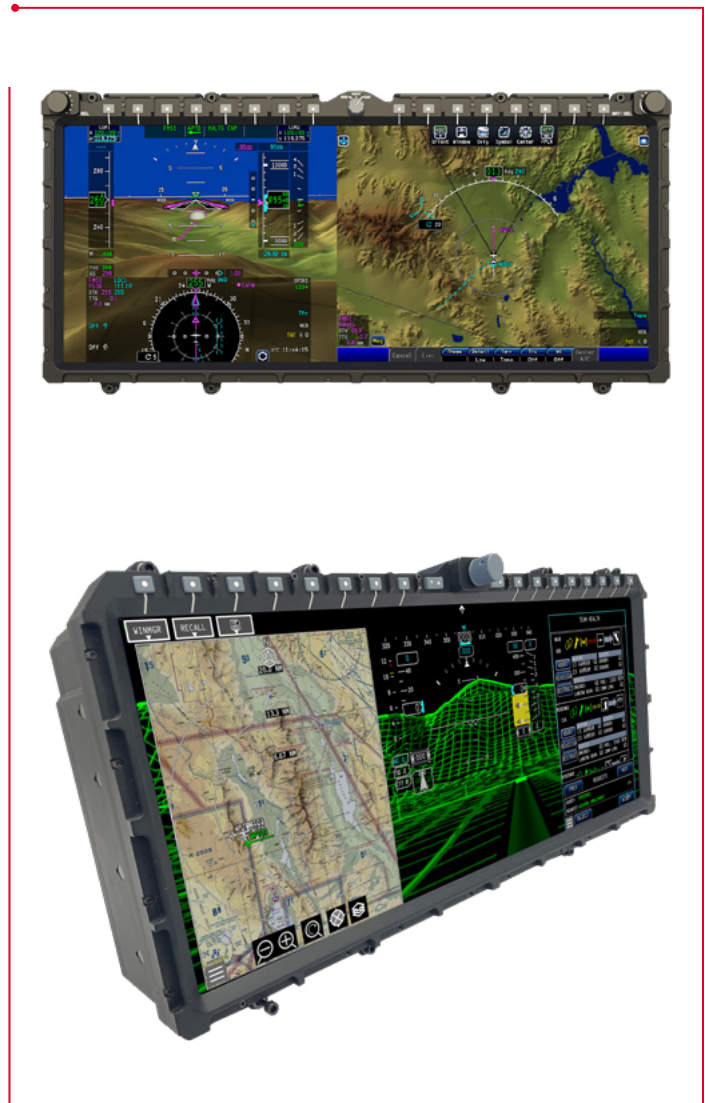
Figure 3 – Configuration files make it easy to flexibly change the application layout of the flight deck to accommodate multiple use cases. These examples show two possible “personalities” for the same large area display (LAD).
